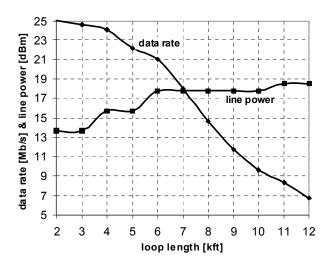
Figure 7: Measured data rate and line power as function of loop length.
