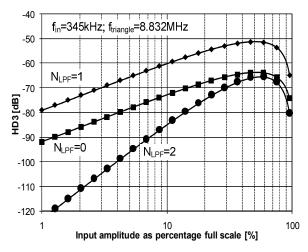
Figure 2: HD3 due to aliasing: theory and simulation (dots).
