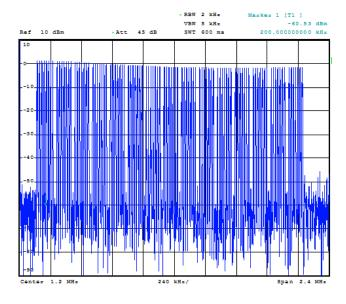
Figure 6: Measured DMT spectrum at line;  $P_{line}=100 \text{mW}$ ; PAR=5.
