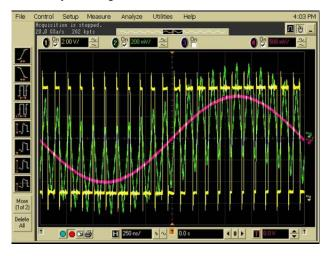
Figure 5: Measured line driver waveforms in one bridge half.
