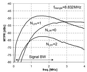
Figure 3: Simulated avg. MTPR due to aliasing; PAR=5.6.
