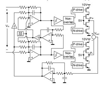
Figure 4: Single-ended representation of line driver.
