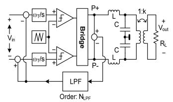
Figure 1: Block diagram of 3-level PWM line driver.
