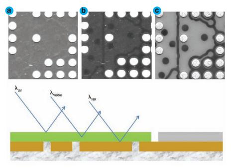
Figure 5. Images of a printed circuit board taken using light sources of various wavelengths: (a) UV at 400 nm, (b) visible using a white LED and (c) NIR at 850 nm. UV light reveals only features on the surface, but not deep inside the board. Copper wires underneath the paint clearly appear in the NIR image, where light with longer wavelengths penetrates more deeply.
