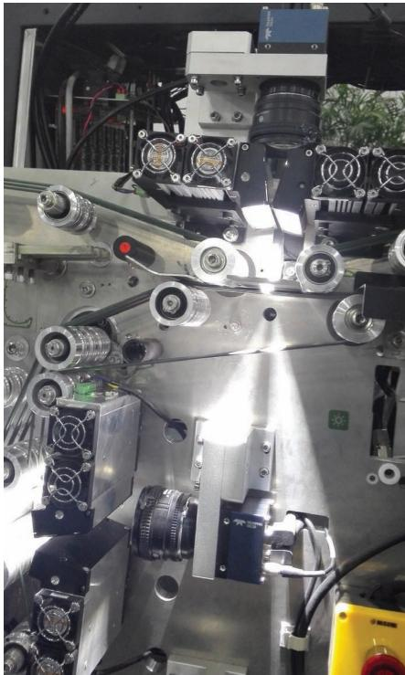
Figure 4. This banknote inspection system uses Teledyne Dalsa's Piranha4 multispectral camera to capture accurate RGB+NIR images at high speed, enabling inspection of both color and NIR images within one camera
