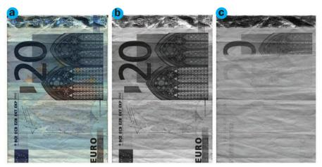
**Figure 3.** A euro banknote image captured by the Piranha4 multispectral camera. Three different outputs: (a) color, (b) monochrome and (c) NIR. Light sources were white LEDs for color and monochrome and 850-nm LEDs for NIR. The image of architectural windows in the banknote was half-printed with IR security inks. The security inks are invisible to the naked eye, as shown in the color and monochrome images. With the NIR light source at 850 nm, the NIR channel unveils these invisible features.
