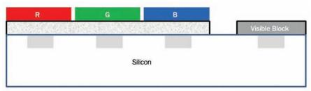
Figure 1. Schematic of Teledyne Dalsa's Piranha4 quadlinear multispectral CMOS sensor using thin-film interference filters. An IR filter blocks color channels, while a visible-block filter passes only NIR wavelengths.
