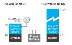
Figure 2: By supporting 64-bit addressing, PCIe can bypass the memory addressing limitations of older 32-bit PCI systems, providing direct access to a virtually unlimited address space with no need for virtual memory.
