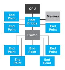
Figure 1: Rather than sharing a set of connections among many peripheral cards as in the traditional PCI bus, PCI Express uses switched serial links to provide a direct, full-bandwidth connection between any two nodes on the bus.
