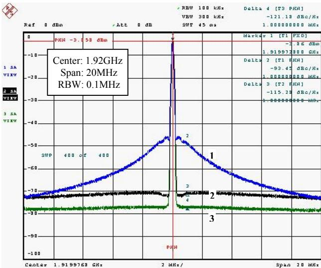
Fig. 8. PLL/DLL output spectrum; the latter with 40/80MHz reference.
