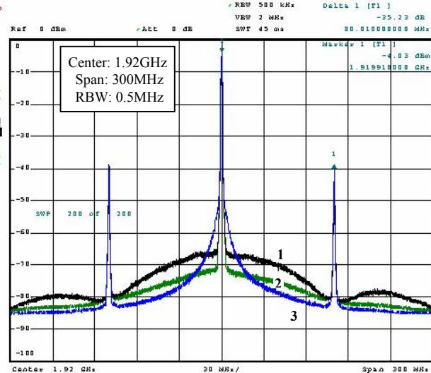
Fig. 7. PLL/DLL output spectrum; the latter with two different REF sources.
