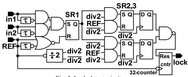
Fig. 5. Lock-detect circuit.
