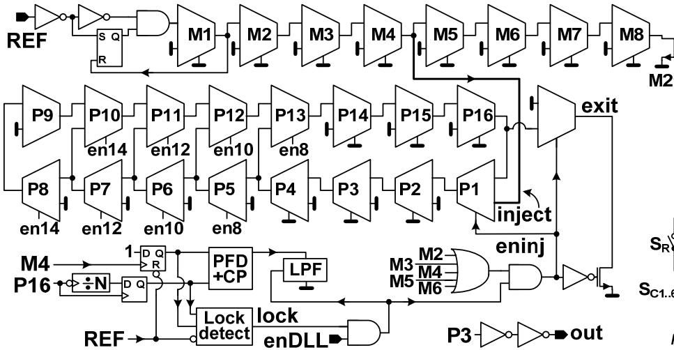
Fig. 4. Schematic of clock multiplier.
