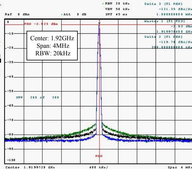
Fig. 9. DLL output spectrum at different loop gains.
