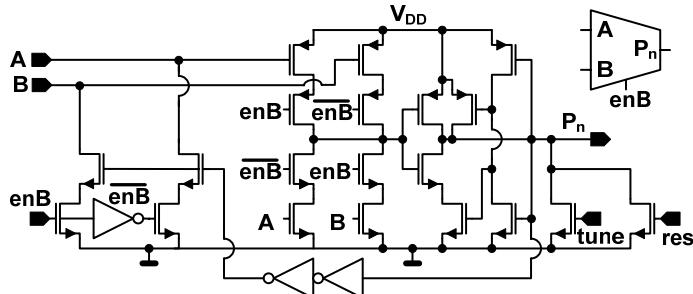
Fig. 2. Schematic of delay stage.
