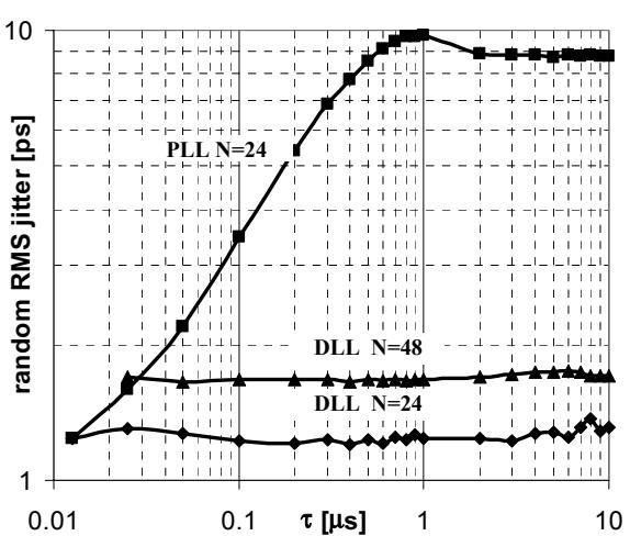
Fig. 11. Random RMS jitter vs. time interval  $\tau$ ;  $f_{\text{out}} = 1.92\text{GHz}$ .
