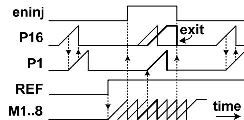
Fig. 3. Waveforms during pulse removal/insertion in DLL mode.
