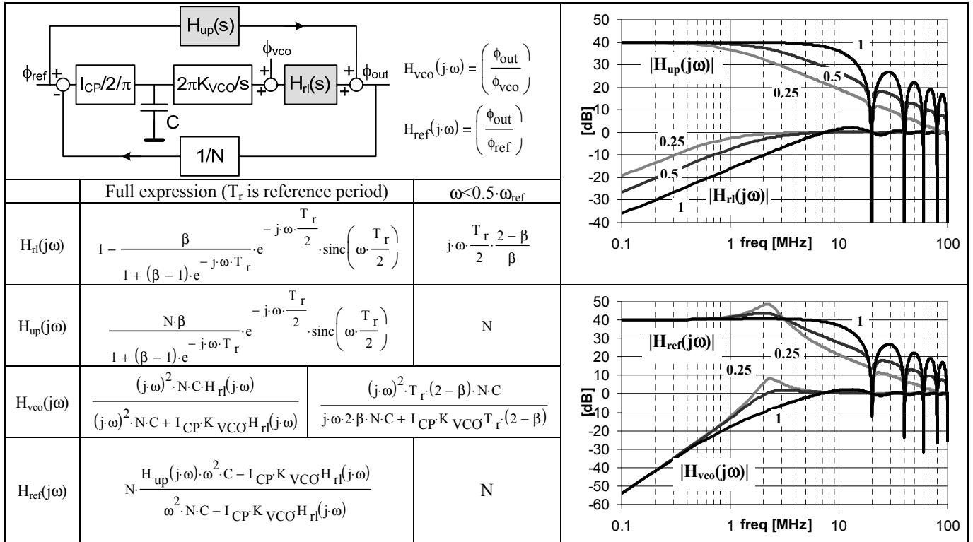
Fig. 1. Freq.-domain DLL model [1] (top left); transfer functions and low-freq. approximations (left); plot of transfer functions for  $\beta=0.25, 0.5, 1$  (right).
