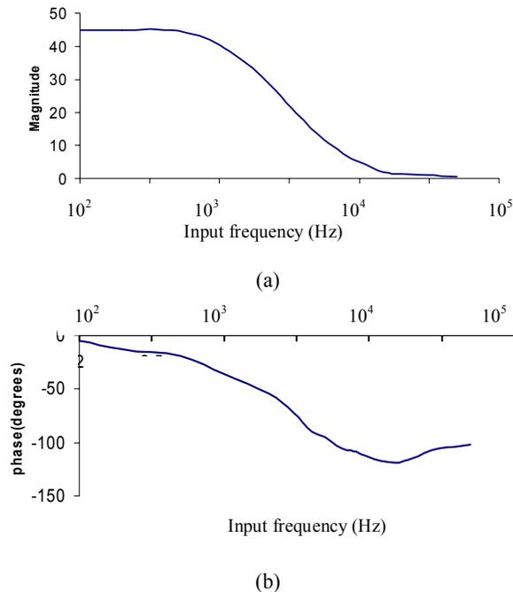
Figure 5: Frequency response of the amplifier (a) Magnitude response (b) Phase response.
