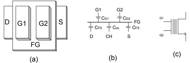
Figure 2: Dual-input FGMOS: (a) Layout, (b) Capacitance model, (c) Symbol
