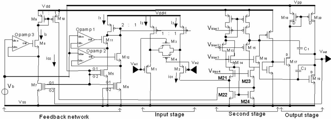
Figure 1: Simplified schematic of the proposed high-voltage amplifier
