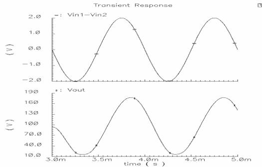
Figure 4: Transient response of a 4V peak to peak differential input sinusoidal signal
