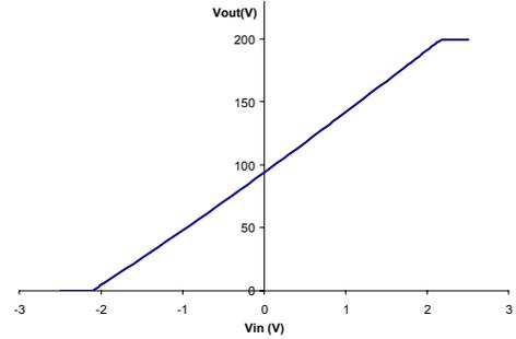
Figure 3: DC sweep of differential input
