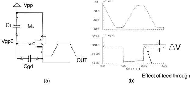
Fig. 5. Effects of feedthrough from the output node: (a) Principle (b) Waveform
