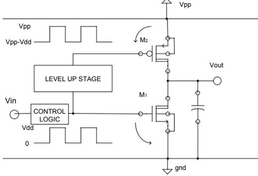
Fig. 2. General architecture of a HV level-up shifter
