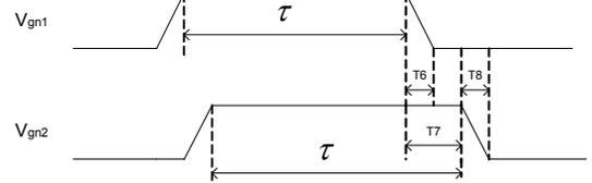
Fig. 7. Timing constraints between  $V_{gn1}$  and  $V_{gn2}$ .
