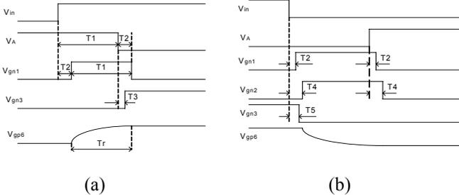
Fig. 6. Waveforms of the control signals: (a) Input rising edge (b) Input falling edge
