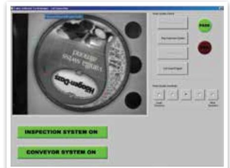
For applications that don't require an HMI, but do require occasional monitoring, the BOA PRO web server provides a run monitor screen that is semi-customizable from the system property page.
