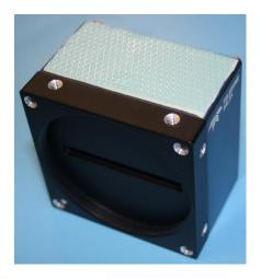
3. Remove the other side film from the gap pad as well. Be careful in that the heat conductive material is a delicate and can be torn off easily.
