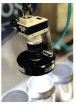
Production-ready system accurately categorized cans as normal or damaged when they were wet or dry. The model proved to be very robust in difficult conditions and could maintain accuracy even with small changes in camera position, focus, and lighting.
