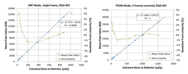
Figure 3 Blue curve shows the sensitivity in DBT (left) and FFDM (right) mode measured at RQA-M2. Green curve shows the deviation from a linear fit through the measurement points.
