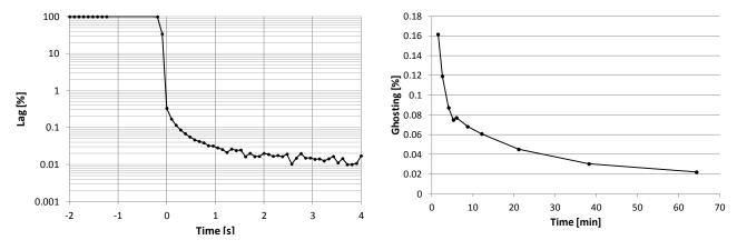
Figure 8 Lag after 3 mGy X-ray exposure during 2s.
