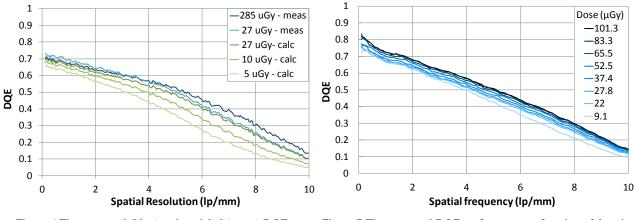
Figure 6 The measured (blue) and modeled (green) DQE performance in DBT mode at RQA-M2.
