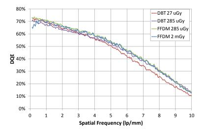
Figure 5 DQE performance at RQA-M2 in DBT mode (single image capture) and FFDM mode (4 frames summed) at typical dose conditions.
