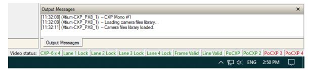
This screen capture shows that the 4 Data Lane signals (i.e. 4 cables) are correct, that Frame and Line Valid signals are active and that cable 1 and 2 carry camera power (POCXP). Cable 3 and 4 do not carry camera power for this Nano model.
