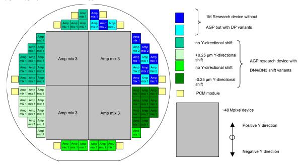
Figure 2: (a) Schematic wafer layout. Different amplifiers – indicated with Amp mix i – and imager configurations are designed. The abbreviations DP and DN stand for the p and n dope implants, respectively.
