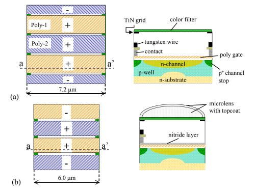
Figure 5: Schematic illustration of the previous (a) and the present (b) pixel architecture. The cross-section is along line a-a'. The 7.2×7.2  $\mu$ m<sup>2</sup> CCD imager [6] operates with three integrating gates (indicated with the + sign) and one blocking gate (- sign), the so-called three-one mode, whereas a two-two mode is used for the 6.0×6.0  $\mu$ m<sup>2</sup> imager.
