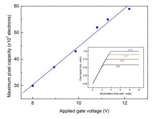
Figure 6: Maximum charge capacity as a function of the applied gate voltage. The inset depicts linearity measurements for different gate voltages.
