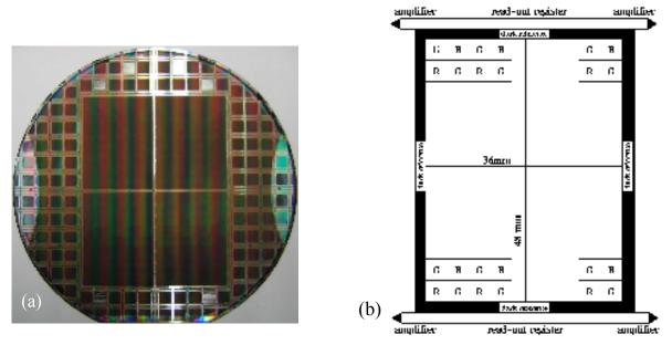
Figure 3: (a) Photograph of a processed wafer using the building block concept, with the layout as depicted by Fig. 2. (b) Schematic layout of a 48Mp full-frame CCD image sensor with Bayer color pattern.
