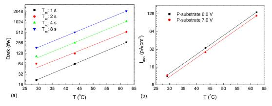
Figure 9: (a) Dark noise (number of electrons) as a function of temperature for different integration times. (b) Dark current as a function of temperature determined for different vertical barrier settings.
