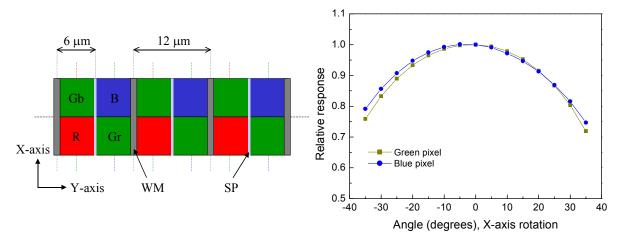
Figure 8: Schematic layout of the pixel design showing the channel stops (SP-lines) and the tungsten bars (WM). The experimental data is obtained for rotation around the X-axis.
