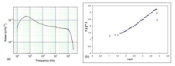
Figure 10: (a) Noise spectrum of the reference on-chip amplifier and (b) the photon shot noise curve, using 6 dB gain and a total integration time of 75 ms.
