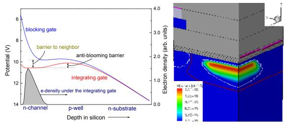
Figure 4: (a) Potential profiles of a filled image pixel with vertical anti-blooming – the blocking and integrating gate – and (b) device simulation of a saturated pixel – one quarter. The pixel architecture is depicted in Fig. 5.
