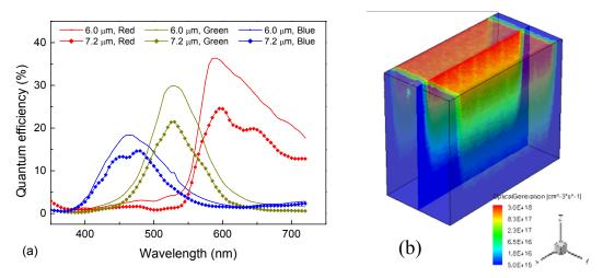
Figure 7: (a) Quantum efficiency spectrum of the  $7.2 \times 7.2 \ \mu m^2$  CCD imager and its  $6.0 \times 6.0 \ \mu m^2$  successor, both with the Bayer color filter pattern. (b) Optical simulation result of half a pixel for a wavelength of 500 nm, within the silicon substrate directly under the gates.
