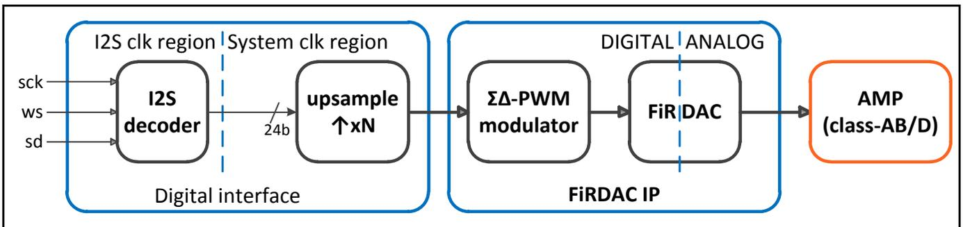
Figure 6 – System overview of the FIRDAC IP for an analog class-D power amplifier
