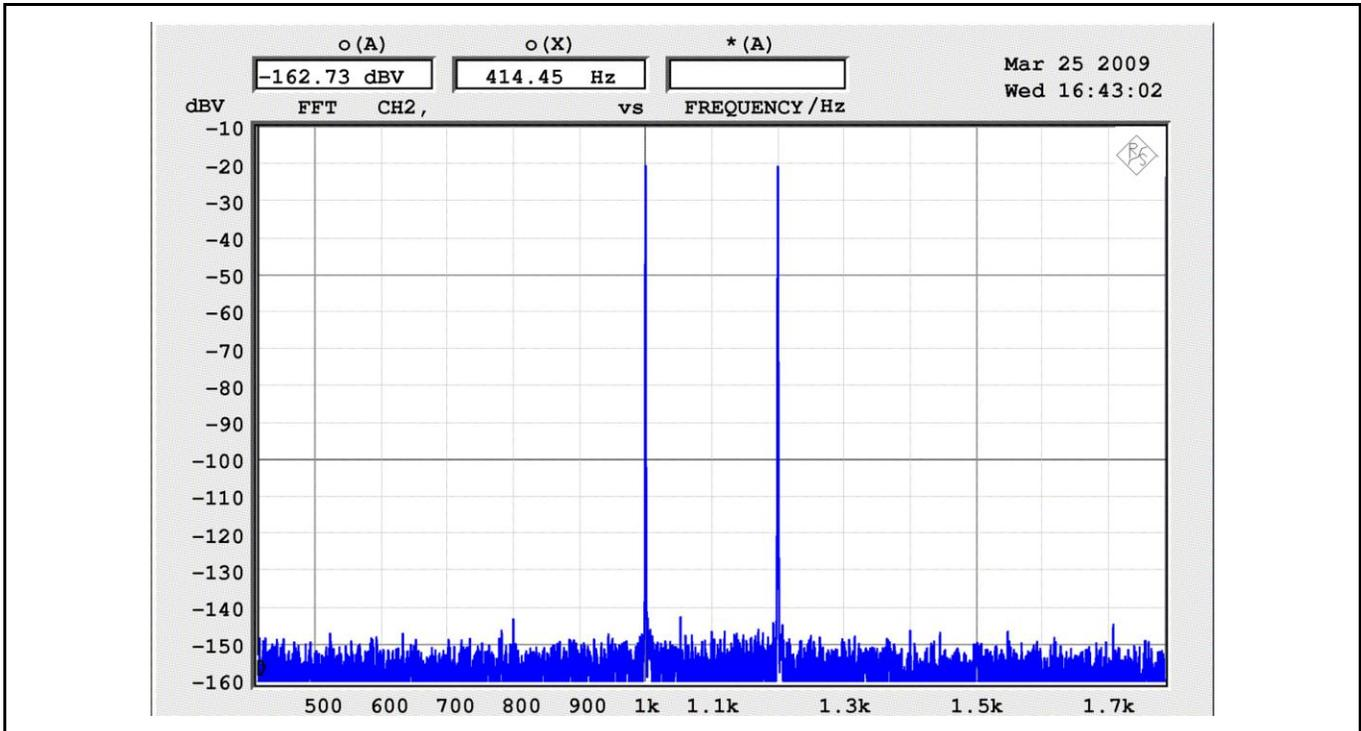
Figure 4 – Two-tone intermodulation 1kHz and 1.2kHz; both input tones at -20dBFS. Intermodulation tone hardly detectable @ 800 Hz.
