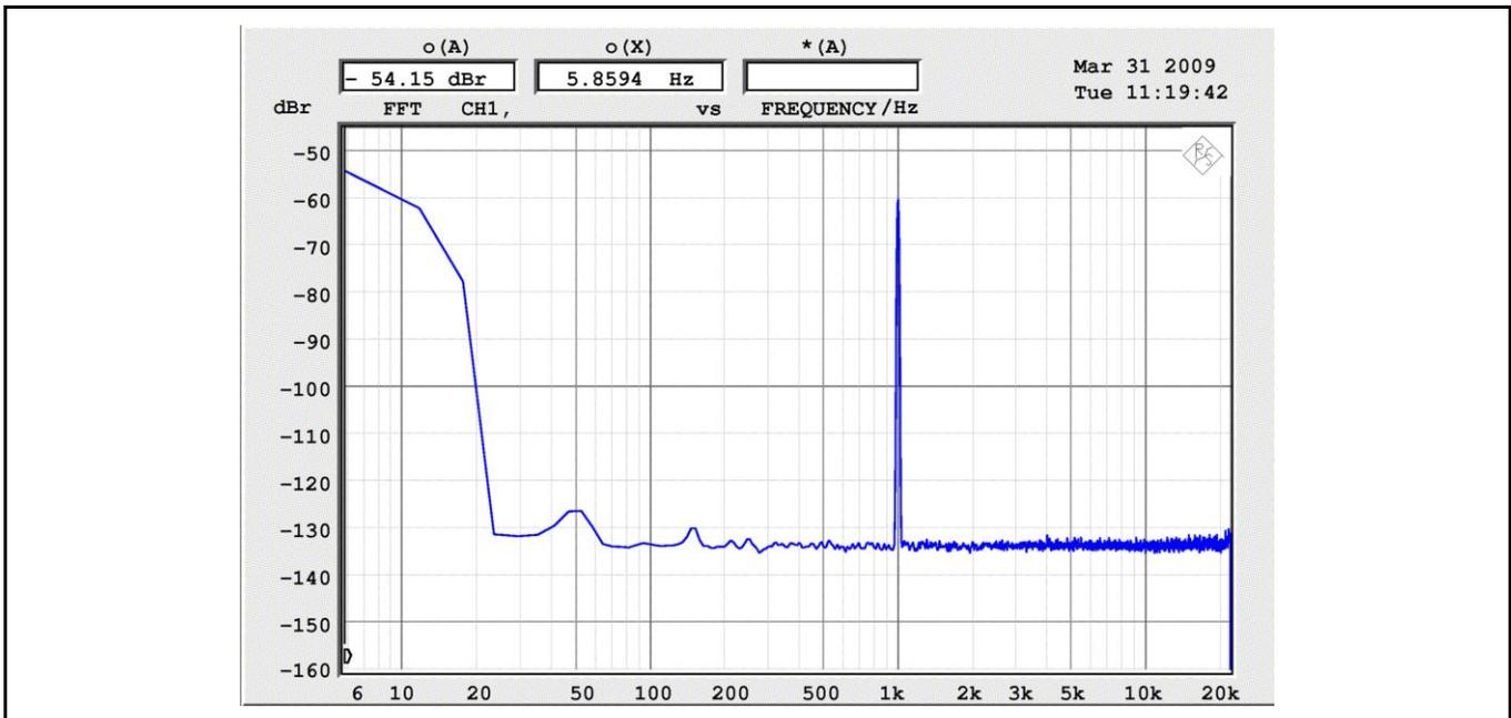
Figure 3 – Output spectrum of the FIRDAC with a single tone of 1kHz
