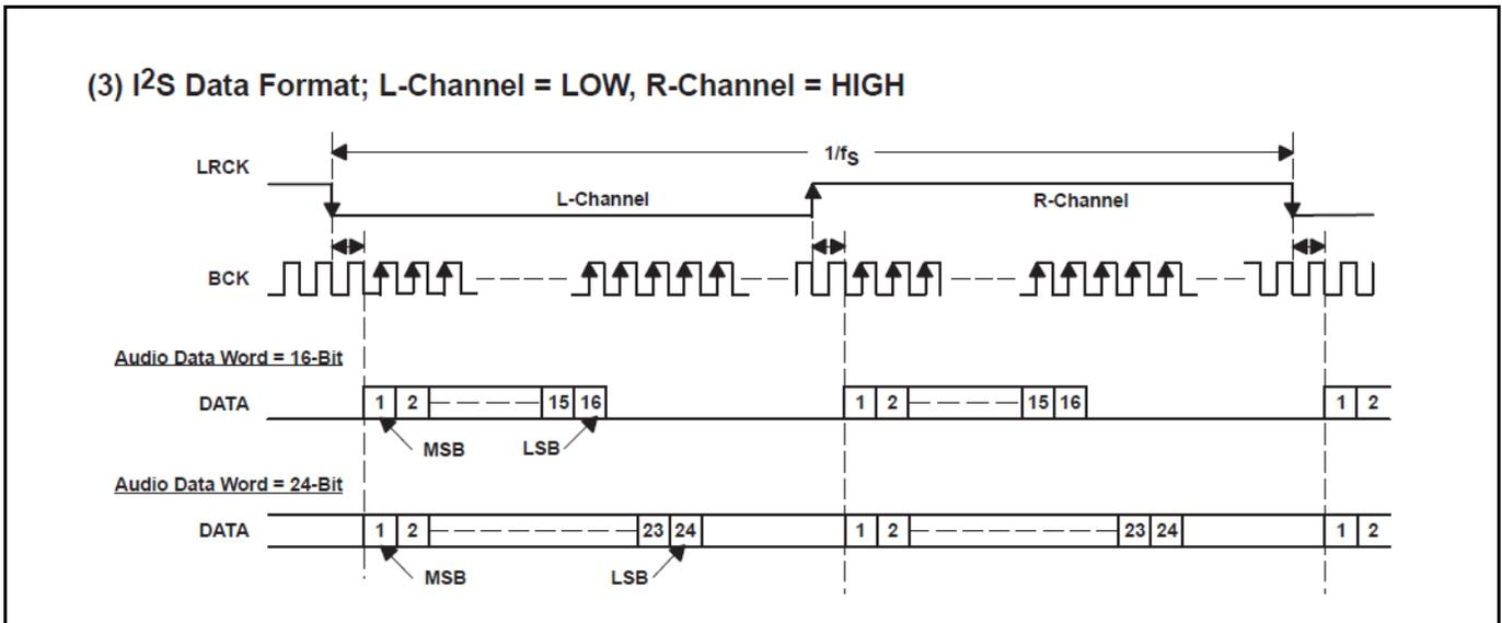
Figure 8 – Audio data interface specification (I<sup>2</sup>S) [PCM1794A]
