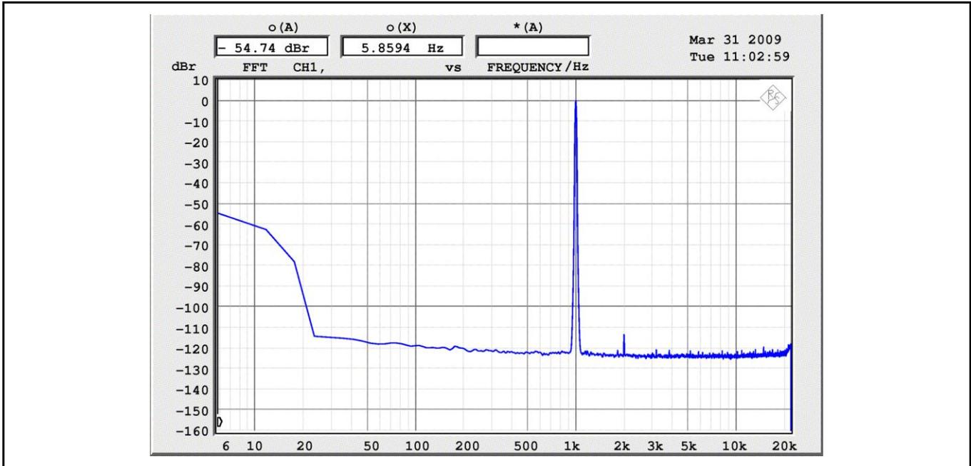
Figure 2 – Output spectrum of the FIRDAC with a single tone @ 1kHz 0dBFS. THD < -110 dBFS.
