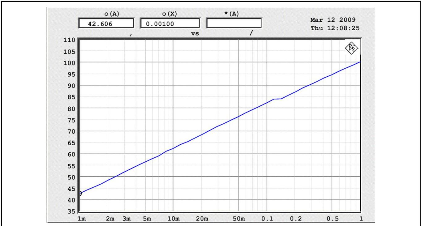
Figure 5 – SINAD vs. input fraction; no weighting filter (irregularity @input 0.12 due to range switching of the audio analyzer)
