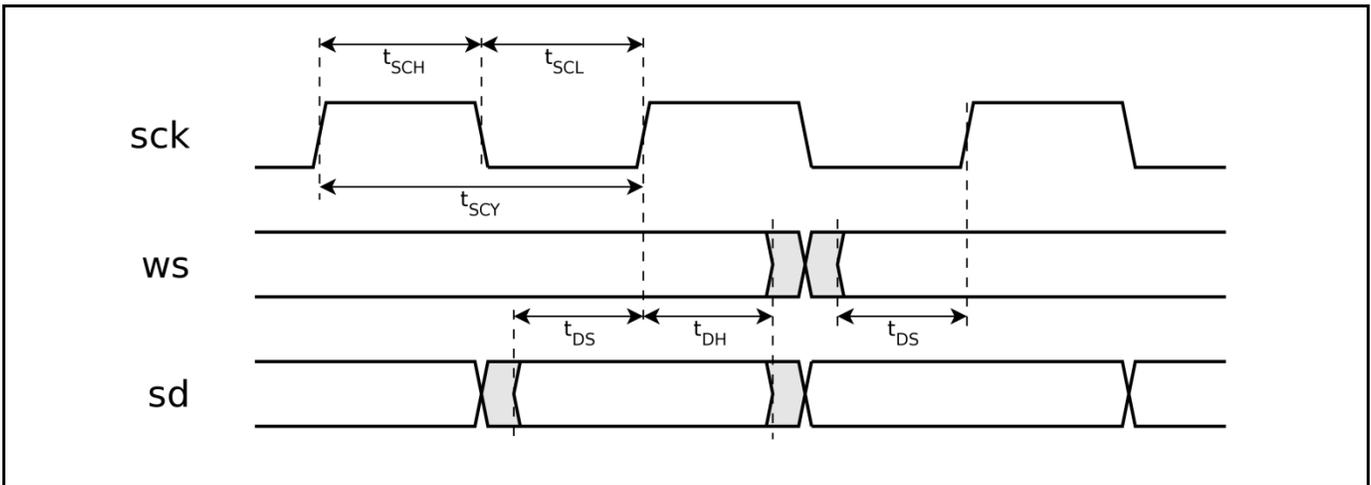
Figure 9 – Audio data interface timing
