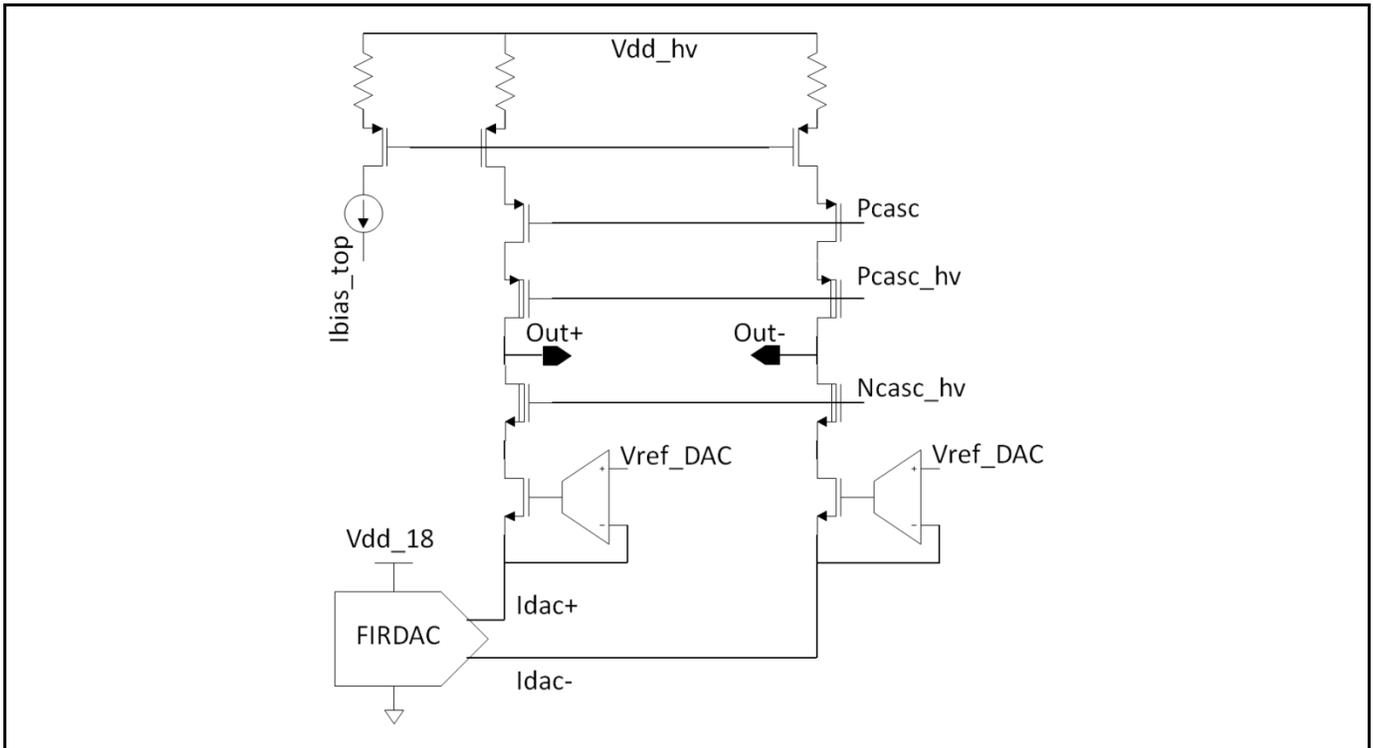
Figure 7 – AXIOM\_PULLFIRDAC applied in the input stage of the linear amplifier
