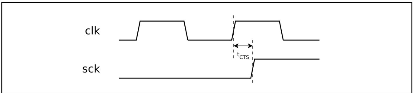
Figure 10 – Definition of clk-to-sck delay
