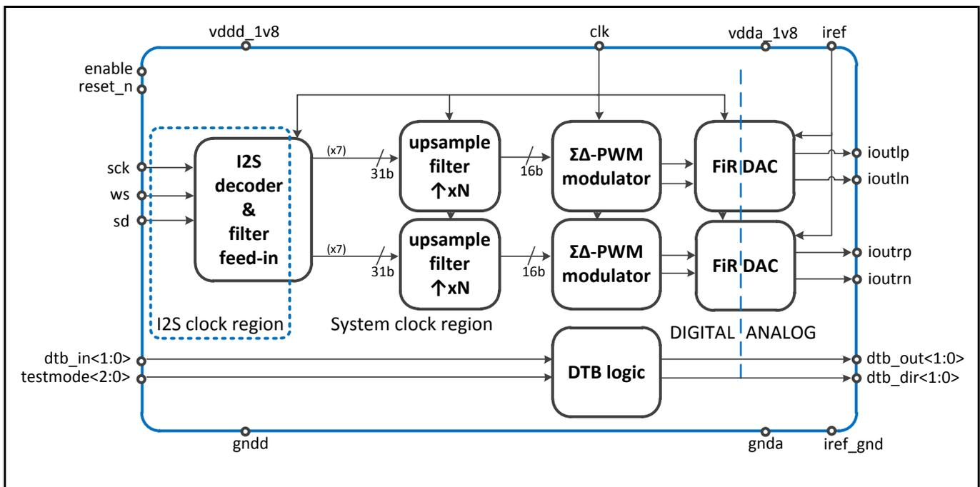
Figure 1 – Block diagram of the FIRDAC IP
