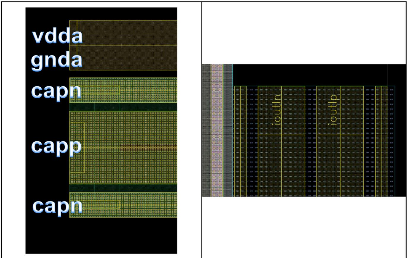
Figure 12 – Layout axiom\_xfabxp018\_pullfirdac detail view of supply pins and output pins
