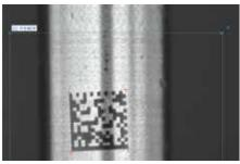
LASER ETCHED 2D CODE ON METAL
