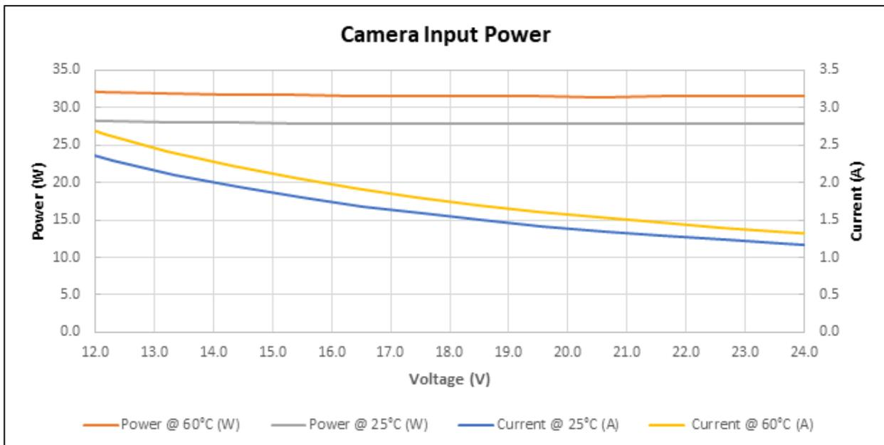
Figure 11: Multifield Model Power Vs. Input Voltage
