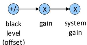
Figure 45: Black Level, Gain and System Gain Processing Chain
