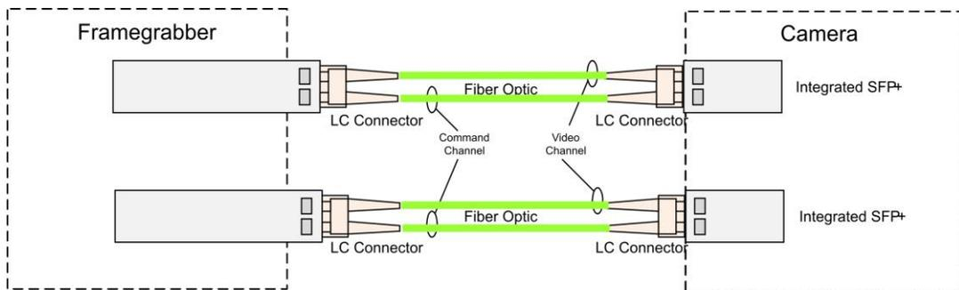
Figure 17: Linea HS Dual LC/SFP+ Connector Configuration
