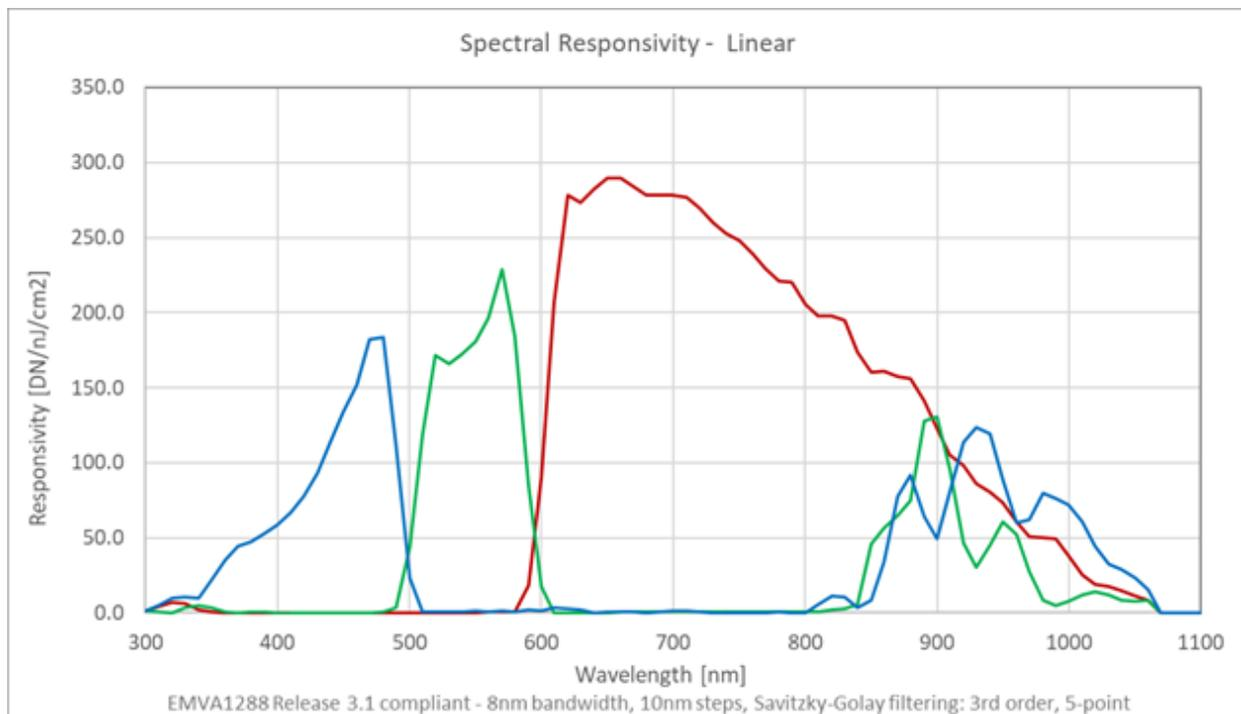
Figure 9: Multifield Model Spectral Responsivity
