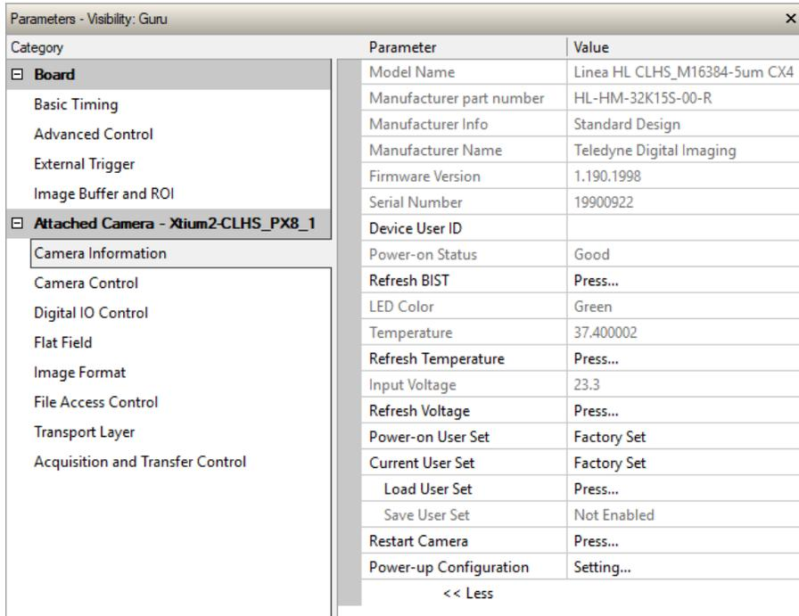
Figure 50: Example CamExpert Camera Information Panel
