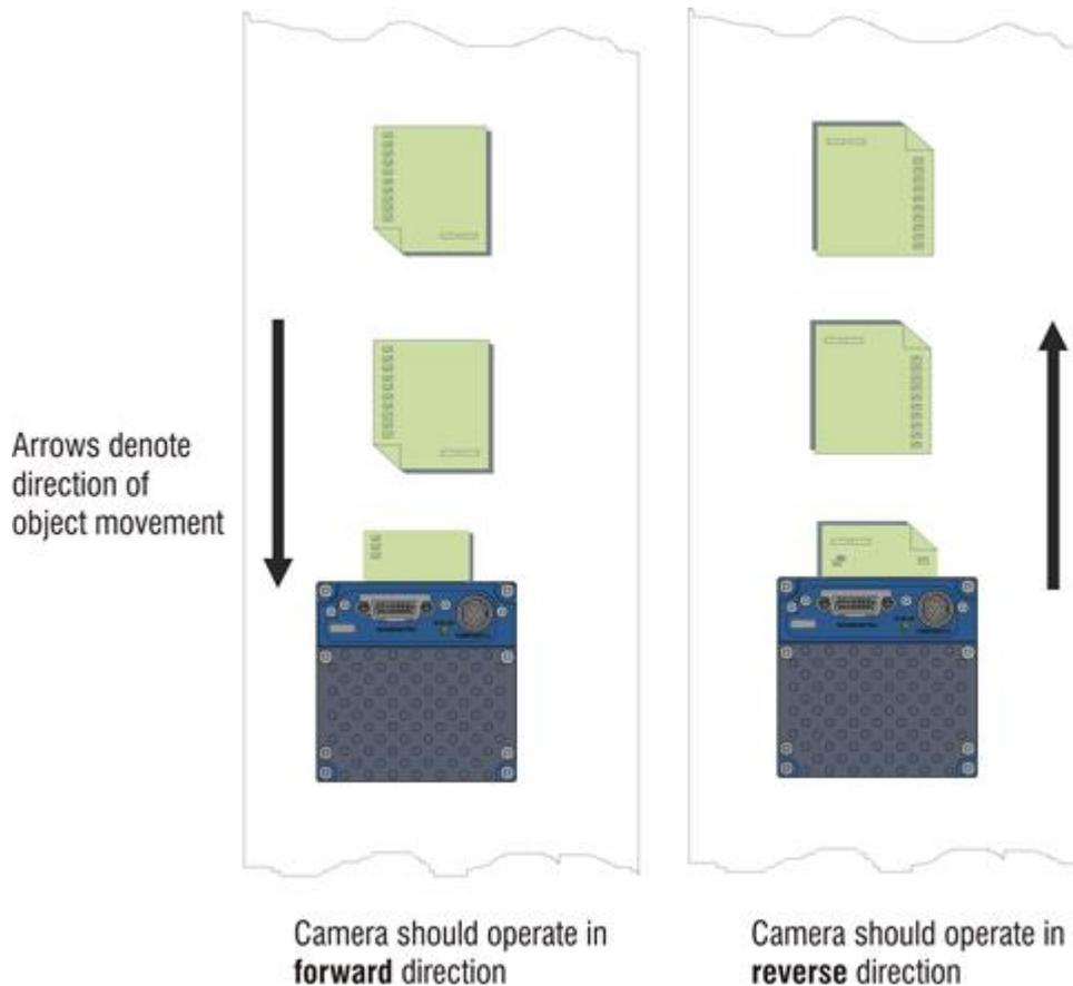
Figure 28: Example of Object Movement and Camera Direction
