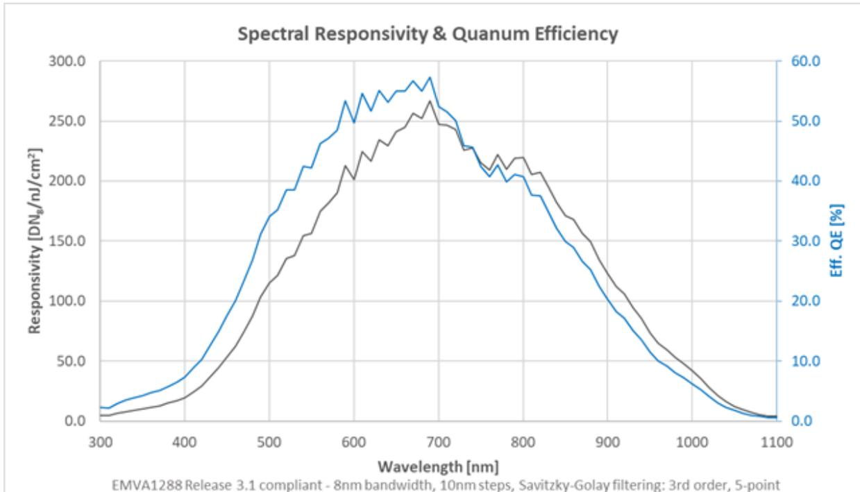
Figure 12: Super Resolution Model Spectral Responsivity & QE, 32k SR Mapped, 1x gain
