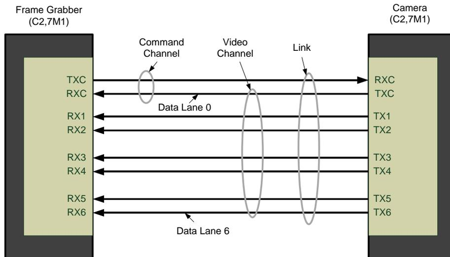
Figure 18: Single CLHS Connector Configuration
