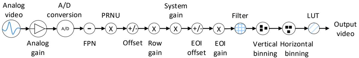
Figure 16: Video data processing chain
