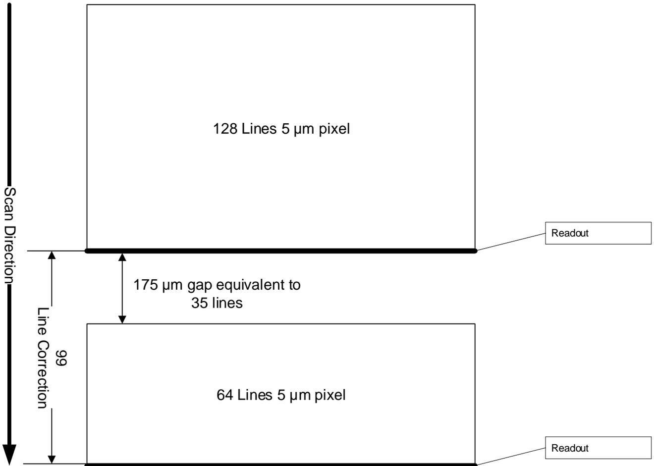
Figure 31: Standard and High-Speed Camera Line Spacing – Reverse Scan Direction
