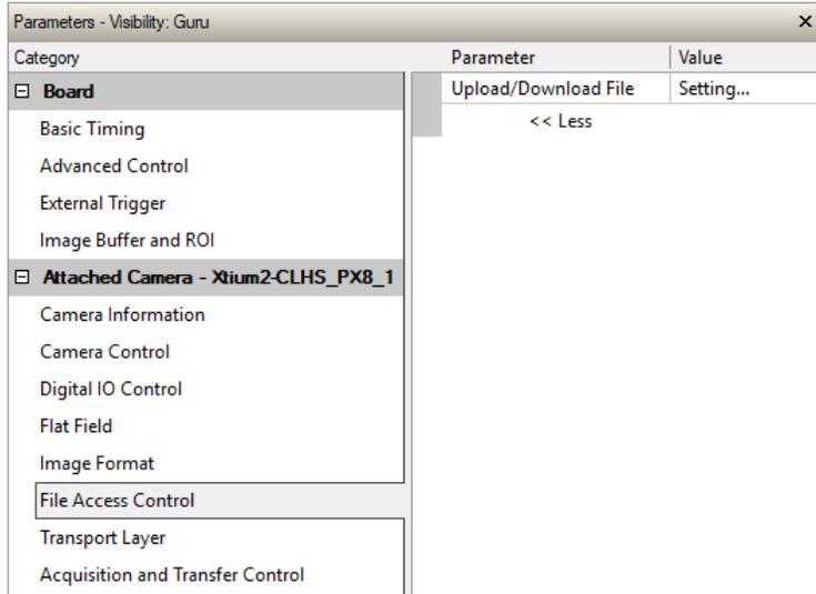
Figure 56: File Access Control Panel
