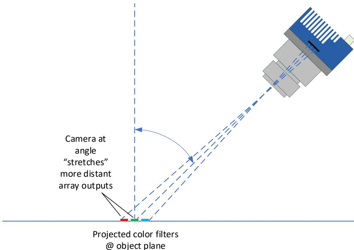
Figure 37: Camera Angle Parallax
