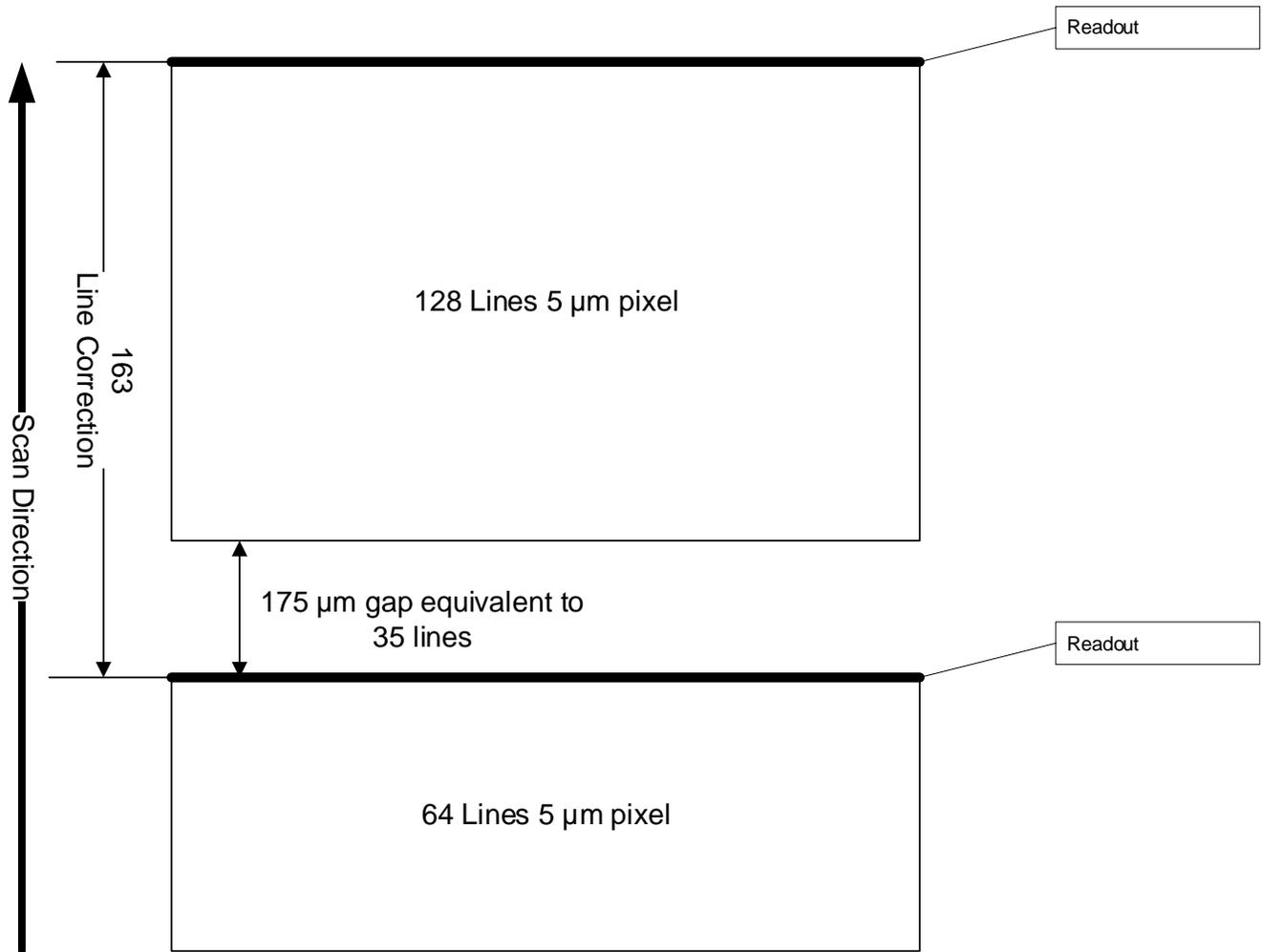
Figure 30: Standard and High-Speed Camera Line Spacing – Forward Scan Direction
