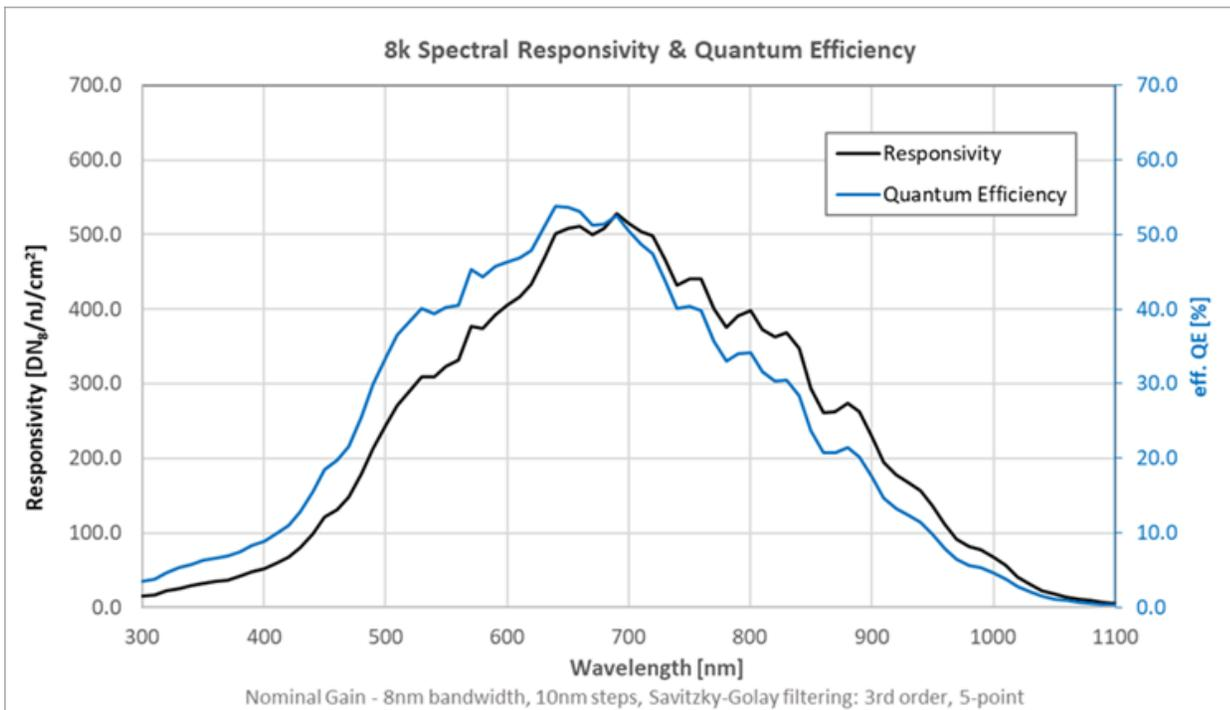
Figure 1: 4K & 8K Monochrome Models Spectral Responsivity & QE
