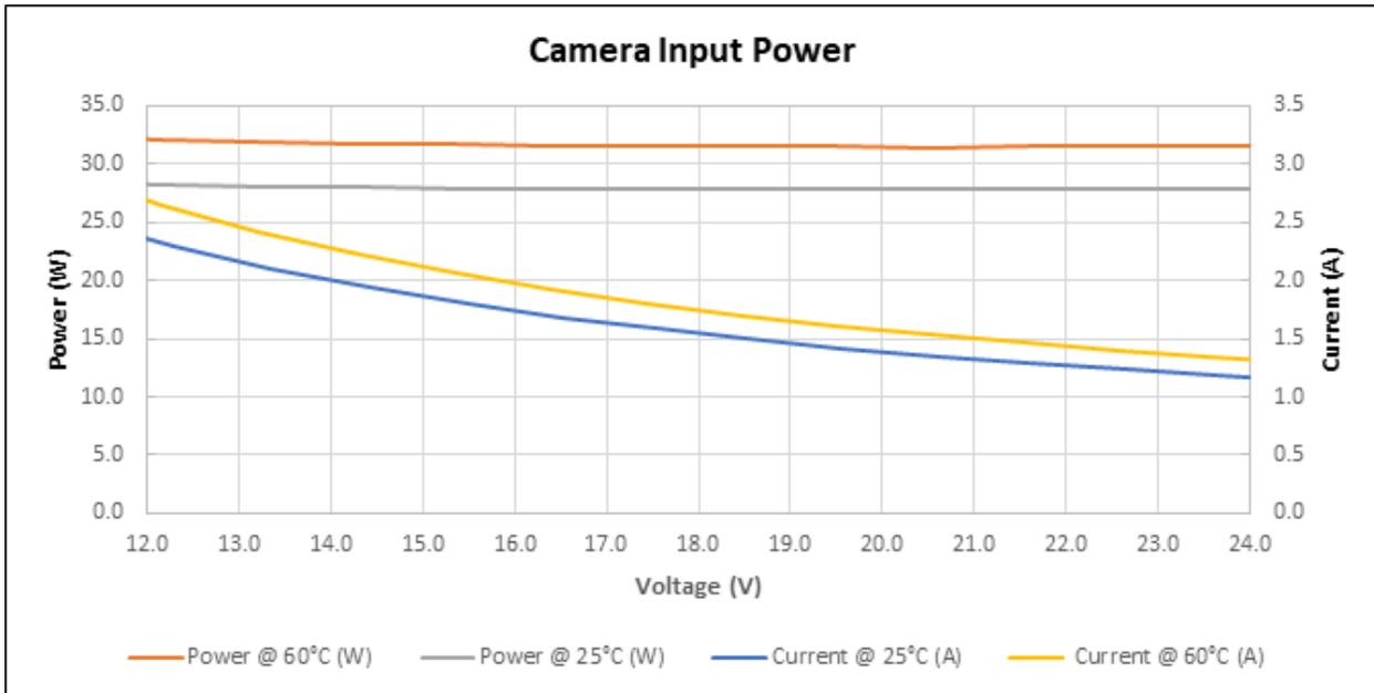
Figure 8: Color Model Power Vs. Input Voltage
