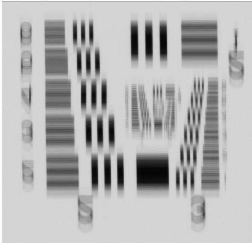
*Figure 27: Image with incorrect scan direction*
