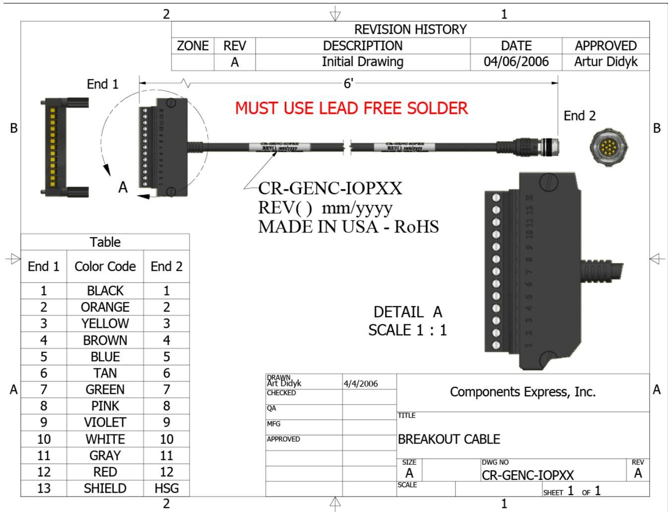
Figure 26: GPIO cable accessory #CR-GENC-IOP00
