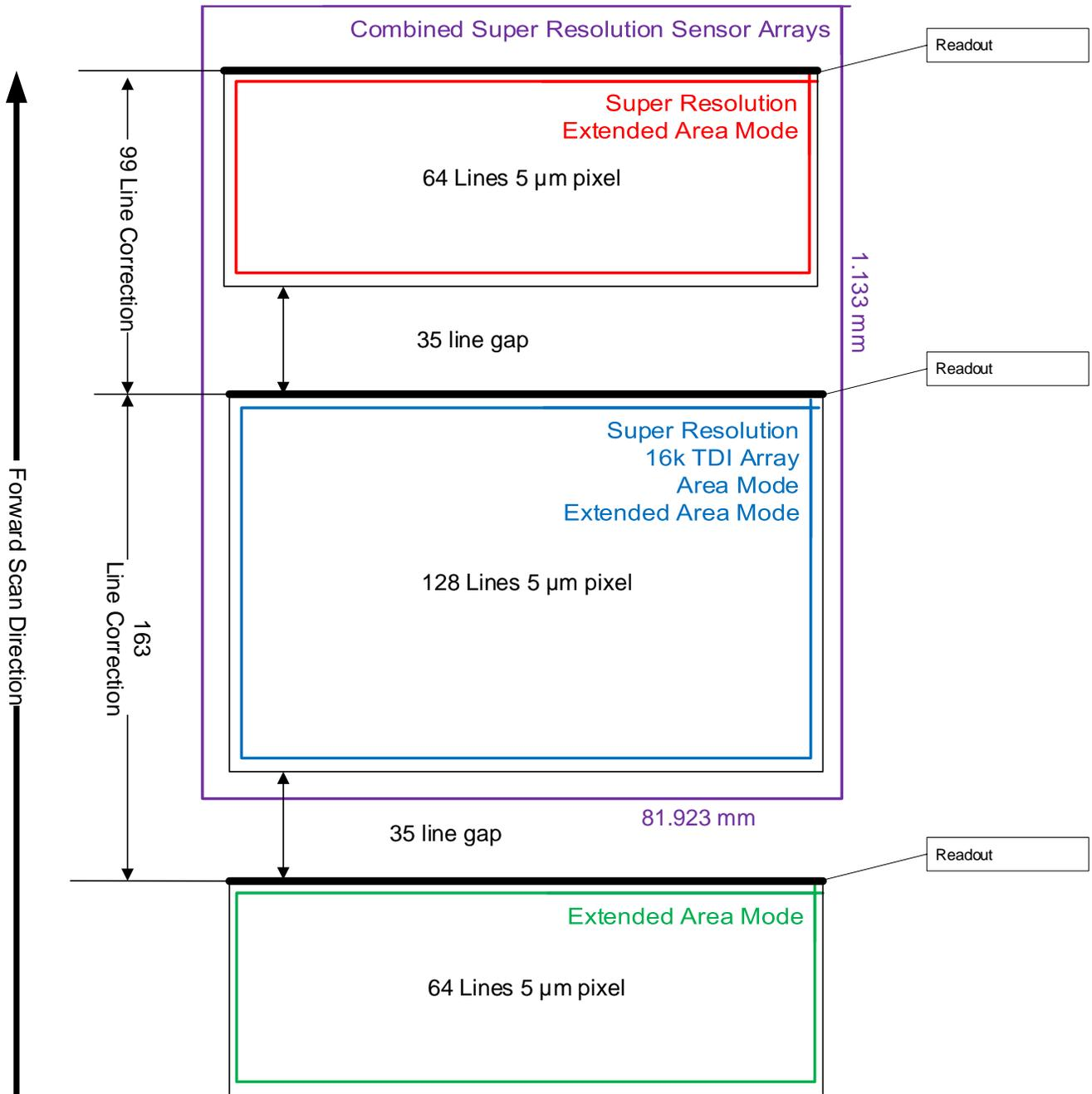
Figure 34: Super Resolution Camera Line Spacing – Forward Scan Direction
