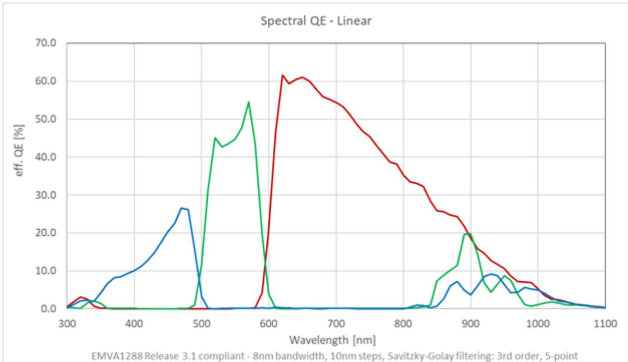
Figure 10: Multifield Model QE
