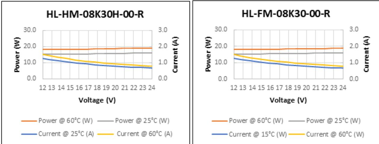
Figure 4: Standard 8K Models (CX4 and SFP+) Power vs. Input Voltage
