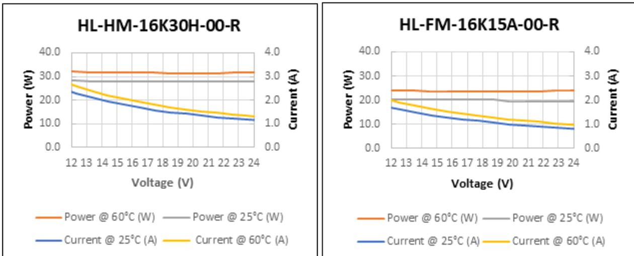
Figure 5: Standard 16K Models (CX4 and SFP+) Power Vs. Input Voltage
