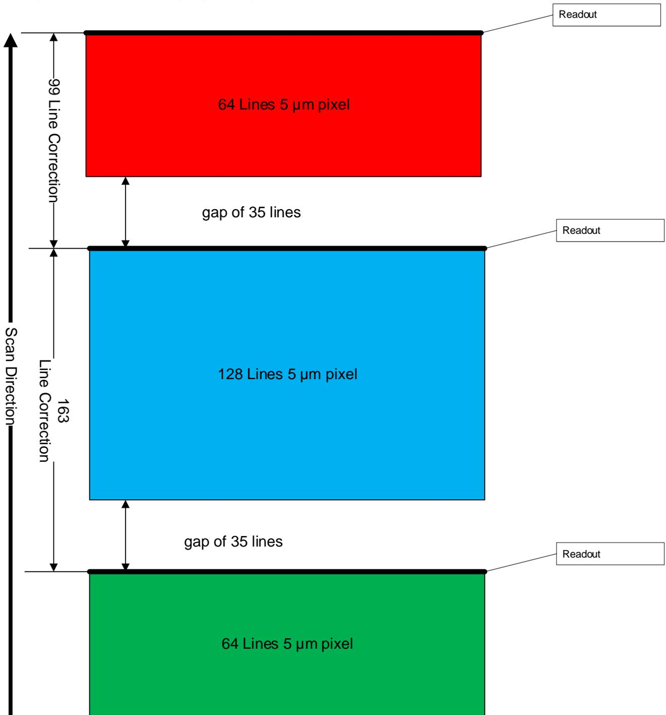
Figure 32: Multifield Camera Line Spacing – Forward Scan Direction
