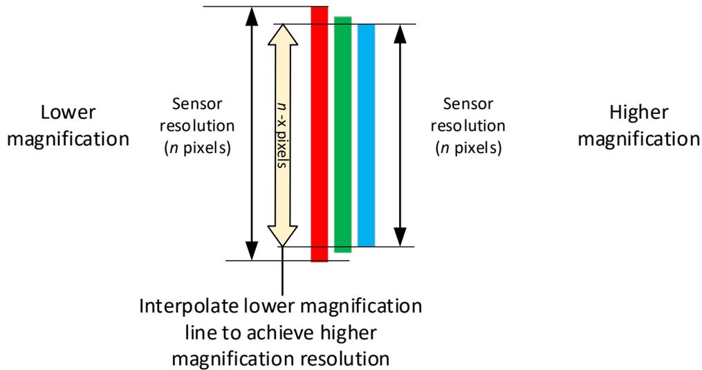
Figure 38: Parallax Effect on Sensor Arrays Output
