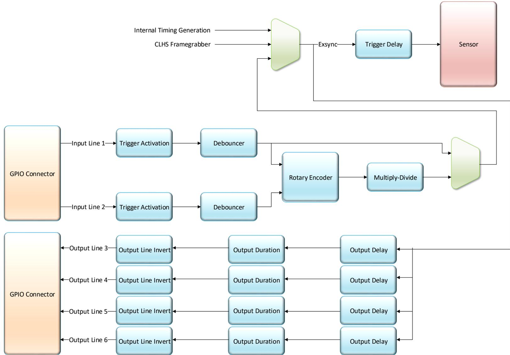
Figure 40: GPIO functionality block diagram
