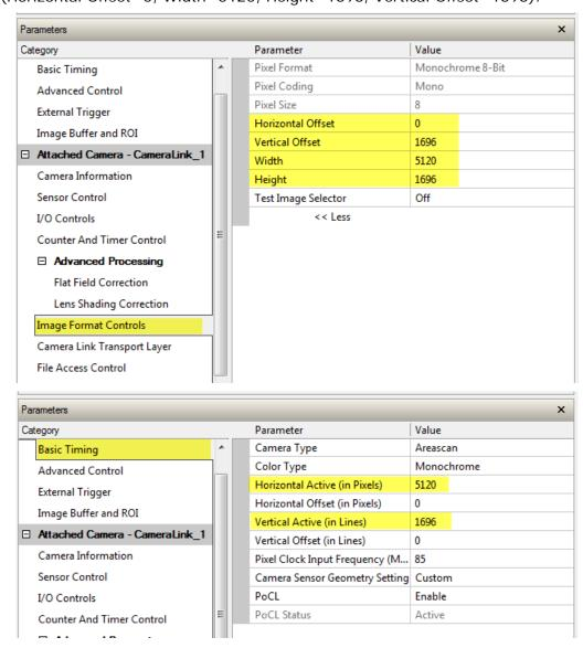
Disable the Lens Shading Correction feature at this time. This must be off for Flat Line calibration.
