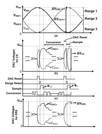
Fig. 2. (a) Input signals,  $V_{INP}$  &  $V_{INN}$  for near Nyquist rate sampling (b) DAC voltages for CS (c) Timing signals for ERS technique (d) DAC voltages for ERS based ADC highlighting the reduction in  $\Delta V_{ERS}$
