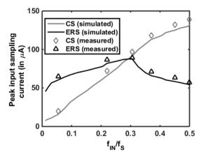
Fig. 5. Peak input sampling current of the ERS and CS based ADCs sampling current profiles as seen in Fig.4 for various input frequencies
