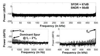
Fig. 7. FFT of the measured ERS based ADC output, normalized to the input tone Fin = 499.96875kHz and Fs = 1MHz.
