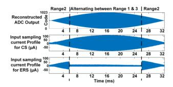
Fig. 4. Measured sampling current profile envelope at Fs-2\*Fin, for both CS and ERS for Fin = 499.96875kHz and Fs = 1MHz.
