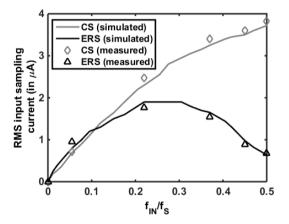
Fig. 6. RMS sampling current of the ERS and CS based ADCs sampling current profiles as seen in Fig.4 for various input frequencies.
