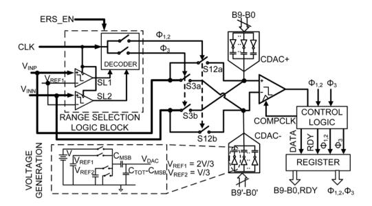
Fig. 1. Charge redistribution SAR ADC Architecture integrated with Energy-Reduced-Sampling technique.
