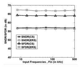
Fig. 8. Comparison of SNDR, SFDR for the ERS and CS based ADCs across input frequencies
