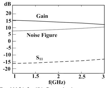
Figure 4.4.4: Gain,  $\mathbf{S}_{11}$  and Noise Figure per channel.
