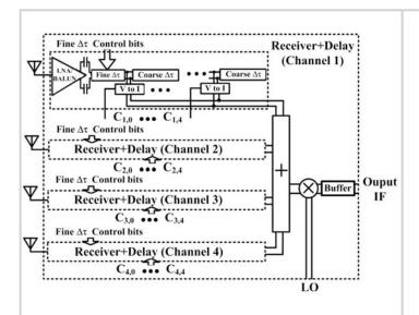
Figure 4.4.1: Block diagram of the 4-channel IC.
