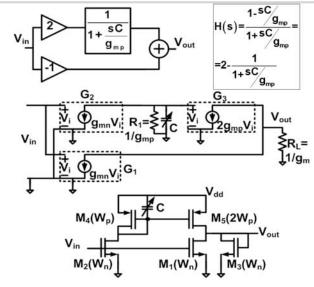
Figure 4.4.2: Delay cell block and circuit diagrams.
