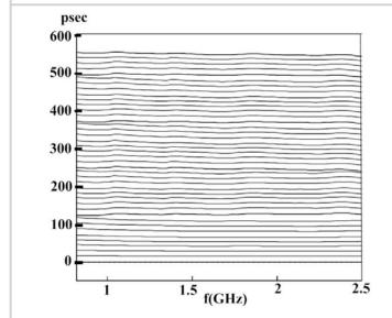
Figure 4.4.3: Measured delay for all delay settings.
