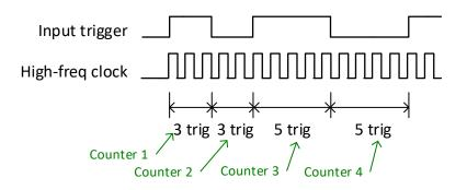
In the above example, the first input period is mapped to 6 (3x2) high-frequency pulses, and the second input period is mapped to 10 (5x2) high-frequency pulses. All pulses' counting is stored in counters cycle by cycle.
