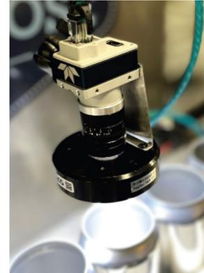
Production-ready system accurately categorized cans as normal or damaged when they were wet or dry. The model proved to be very robust in difficult conditions and could maintain accuracy even with small changes in camera position, focus, and lighting.
