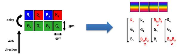
This color mode ( $5\mu m$ ) requires the indication of "Forward/Reverse" to the camera in order to manage the delay between the two coloured lines.
