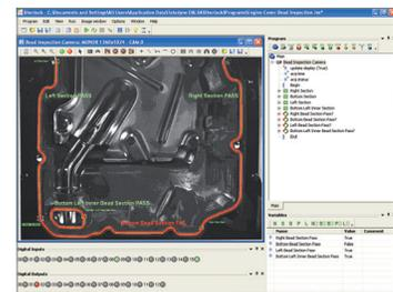
Sherlock offers flexible camera interfacing, together with a rich suite of vision capabilities that can be applied to the most challenging of applications. Sherlock supports advanced scripting, custom operator interface design and the inclusion of 3rd party proprietary algorithms.
