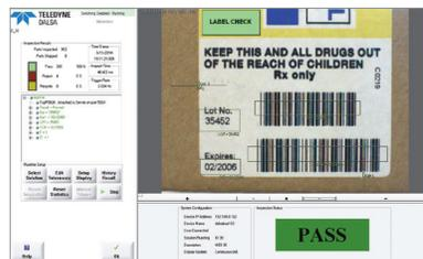
iInspect Express supports applications that use up to 8 cameras of the same type. The interface has been designed to allow setup and deployment of solutions with little or no prior vision experience. iInspect Express provides a common set of tools and capabilities that are relevant for most applications and industries.
